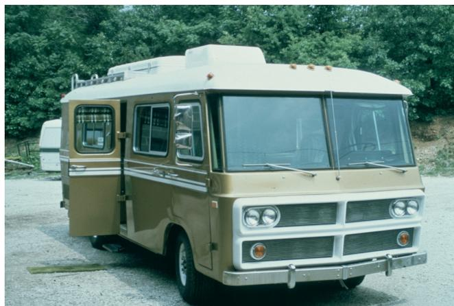
The original Cortez Motorhome from 1964. The Clark Forklift Company began making these small motorhomes in 1963 in Battle Creek, Michigan, and are commonly referred to as Clark Cortez motorhomes. Class-A motor coaches are built as an integrated unit, including the chassis and engine, whereas Class-B and C motorhomes are built on top of an existing truck chassis.
