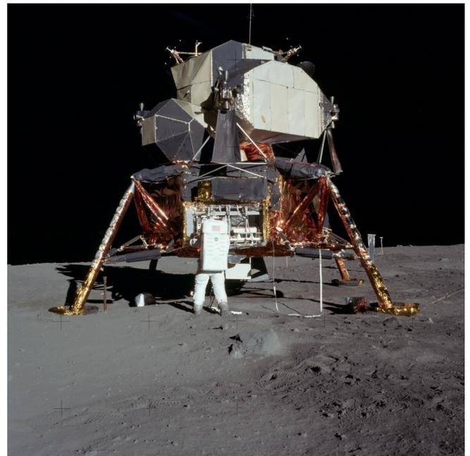
Buzz Aldrin removing the passive seismometer from a compartment in the SEQ bay of the Lunar Lander, 21 July 1969.
