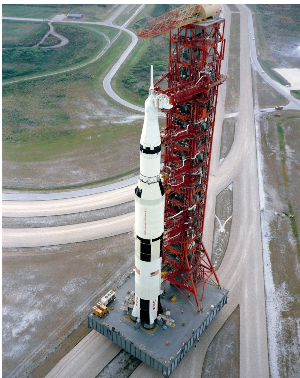
The Saturn V stack and its mobile launch tower are atop a huge crawler-transporter at the Rollout of Apollo 15 -11th May 1971
