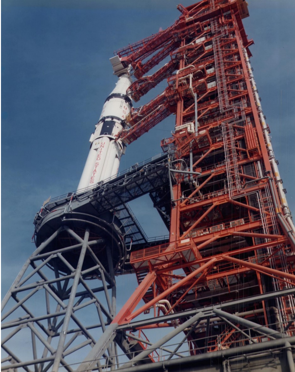
A Saturn Ib with the Skylab 4 Mission on the Milkstool at the LUT.
