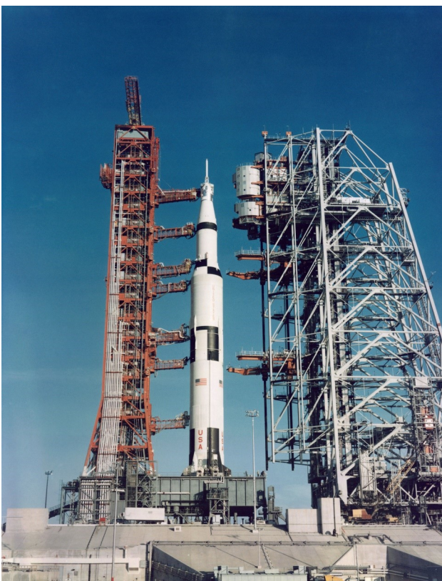
S68-55424 (17 Dec. 1968) --- Ground-level view of the Apollo 8 (Spacecraft 103/Saturn 503) space vehicle at Pad A, Launch Complex 39, Kennedy Space Center (KSC). The Apollo 8 stack was photographed during a pre-launch alert-mobile service structure pull back. (Mobile launch tower on left and mobile service structure on right.) Credit: NASA
