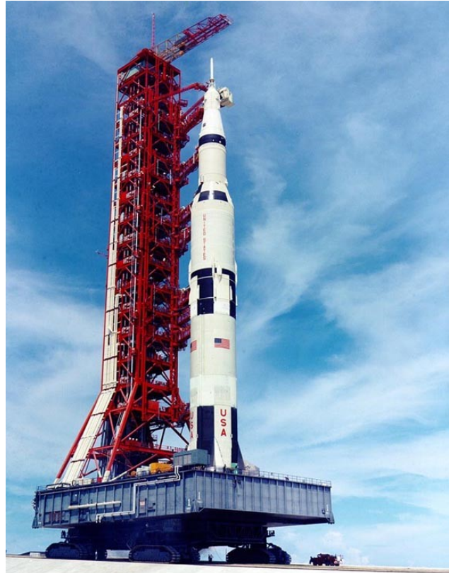
The First: Mobile Launch Platform with the new Launch Umbilical Tower and the Saturn V launcher of Apollo 4, all carried towards Launch Pad 39a atop the Nasa crawler, 19th June 1967 .
