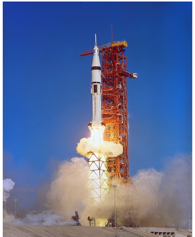
Boosted aloft atop a Saturn IB rocket, and utilizing a special "milk stool" to raise its umbilical connections to the proper levels on the Pad 39B gantry, the third and final Skylab crew takes flight on 16 November 1973. Credit: NASA
