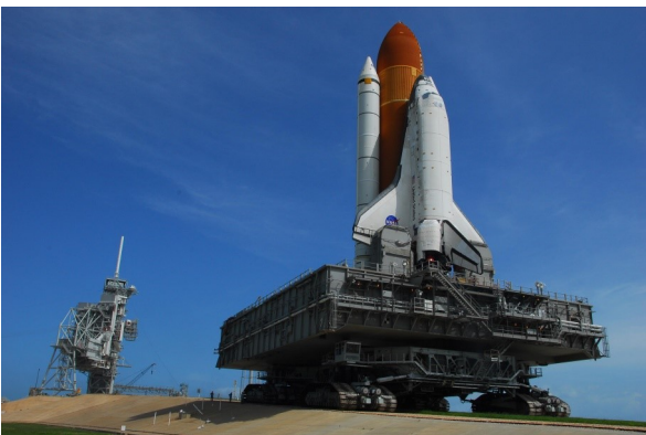
Above: Space Shuttle Discovery climbs the five percent grade to the top of the hardstand at Launch Pad 39A. Rollout is a milestone for the STS-120 mission to the International Space Station.
