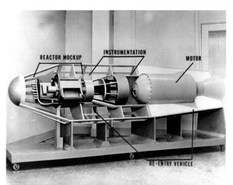
Mockup of the fourth stage of the Scout launch vehicle which launched the re-entry vehicle, including a reactor mockup,
