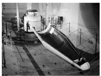
Researchers at the National Aeronautics and Space Administration (NASA) Lewis Research Center conducted a series of shroud jettison tests for the second Orbiting Astronomical Observatory (OAO-2) in the Space Power Chambers during April 1968. Credit: NASA
