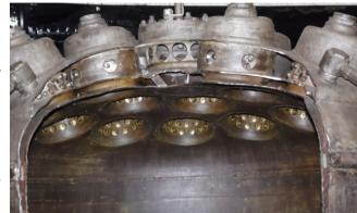
Detail of the A4's rocket engine showing the multitude of injection chambers and double wall construction. Credit: Wikimedia Commons/Skipweasel, 2018
