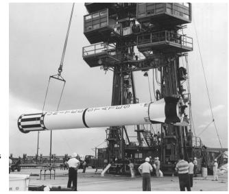
The Mercury-Redstone booster for flight Mercury-Redstone 4 (MR-4) is here being erected on the launch pad. Photo published on July 16, 1961, but probably taken much earlier, since the booster was normally erected weeks before the launch date. Credit: NASA
