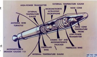
Schematics for "Explorer 1", the first satellite successfully launched by the USA. Credit: NASA
