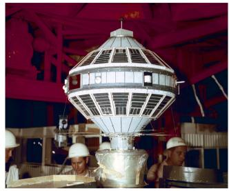
Juno II was a part of America's effort to increase its capability to lift heavier satellites into orbit. One payload was Explorer VII. This photograph depicts workers installing the Explorer VII satellite on Juno II (AM-19A) booster. The Explorer VII investigated energetic particles and obtained data on radiation and magnetic storms.
