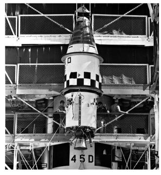
Agena A upper stage with Bell Model 8048 rocket positioned on top of an Atlas rocket at Cape Canaveral, ahead of the May 1960 launch of MIDAS-2 Credits: US Air Force
